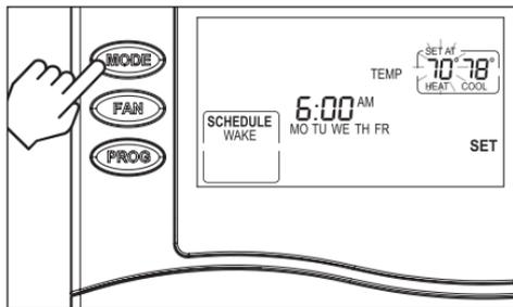
4. Press **MODE**, COOL setting flashes. Press **▲** or **▼** to adjust the cool setting.
